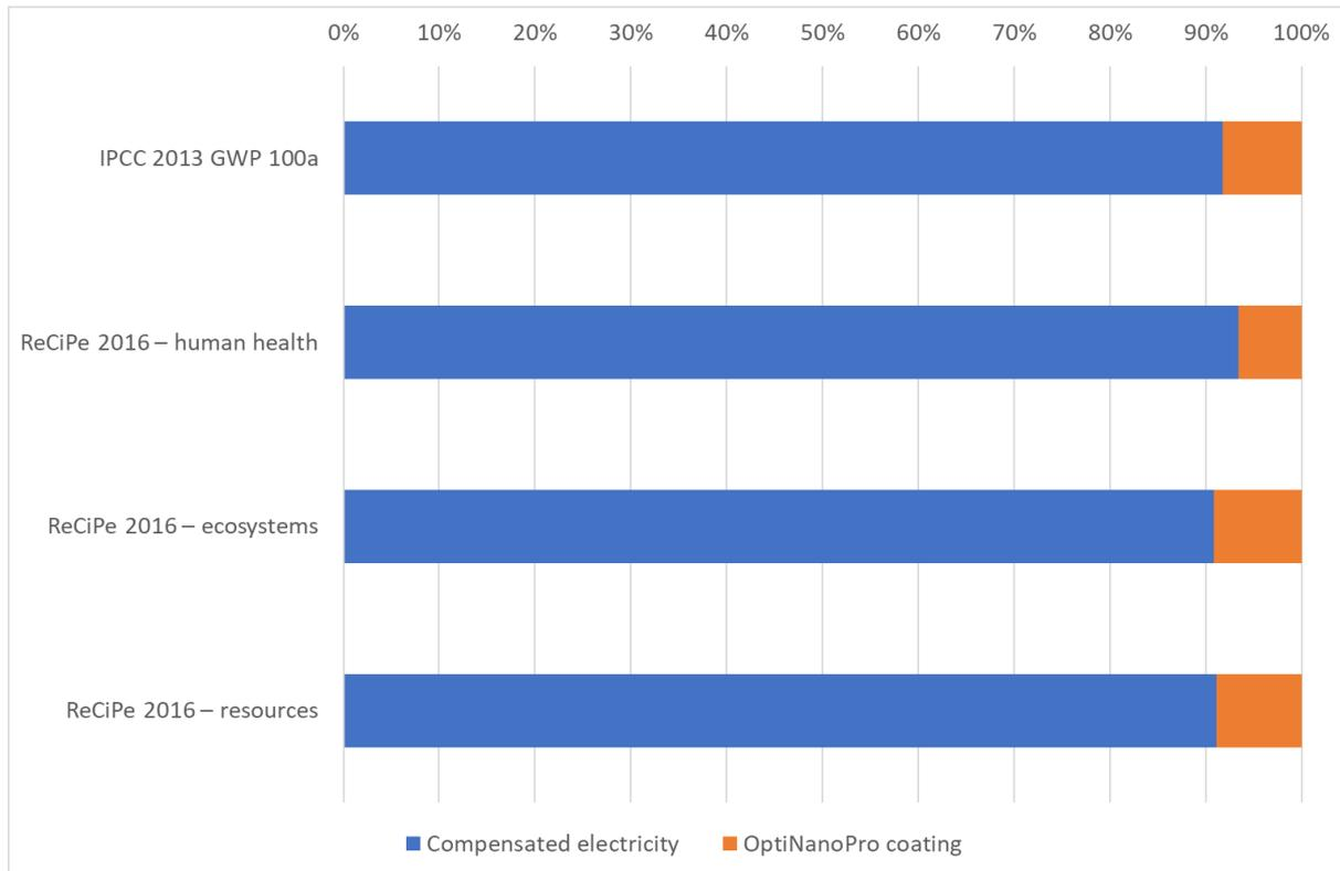
Figure 8: Hotspots of the environmental footprint when coated OPV cells produce 5% less electricity
