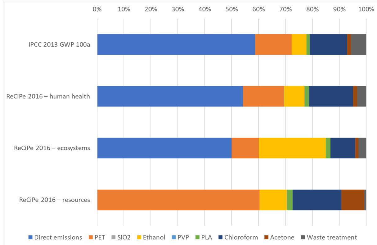
Figure 9: Hotspots of the environmental footprint of the production and waste treatment of the OptiNanoPro coating
