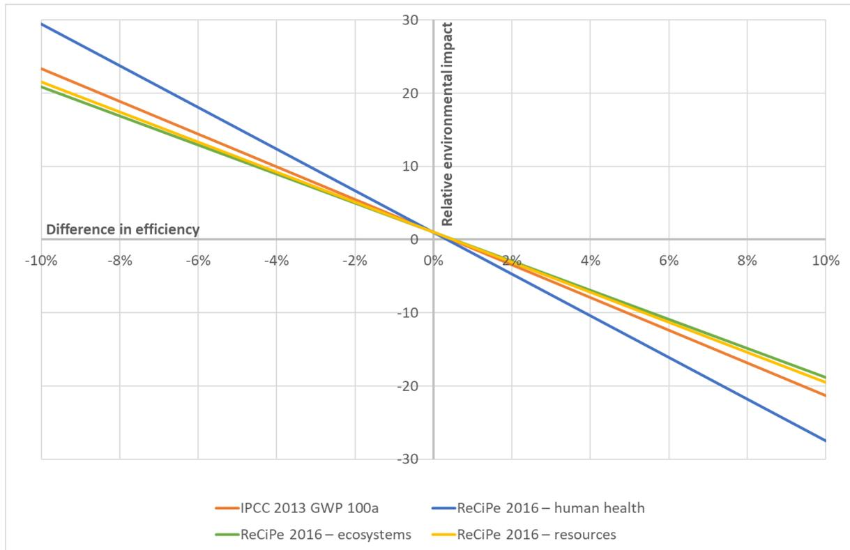
Figure 1: Environmental impact of the OptiNanoPro self-cleaning coating for OPV panels, relative to uncoated cells (/m<sup>2</sup>)
